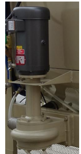
100 Mesh Abrasive Suspension with 3 HP
