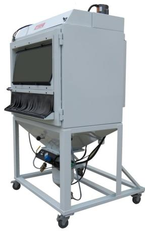
Side to side Sandcarving on large panels with a unique operator blast station including the vacuum operated slit-rubber curtain over brushed port
