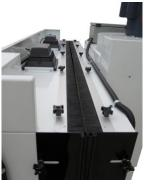
Right and Left Side Opening with adjustable panels, Top Opening Brush Sealed...Advanced LED Cabinet Lighting with attached 440 Sq.Ft. Cartridge Dust Collector
