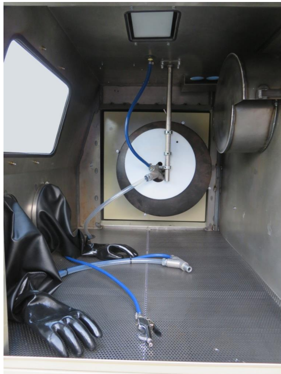
N-200 showing TB-2 with offset manual blasting station and optional pop out shield.
